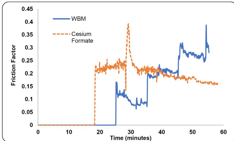
Figure 5—Friction factor profile of an inhibitive mud (Cesium formate) and a conventional water-based mud.
