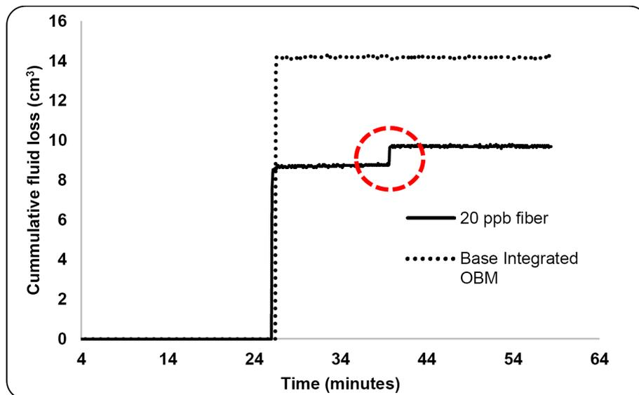
Figure 9—Dynamic fluid invasion profile for base integrated OBM and 20 ppb fiber LCM.
