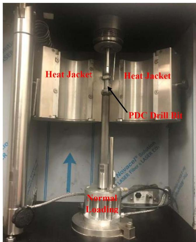
Figure 1—High pressure high temperature drilling simulator
