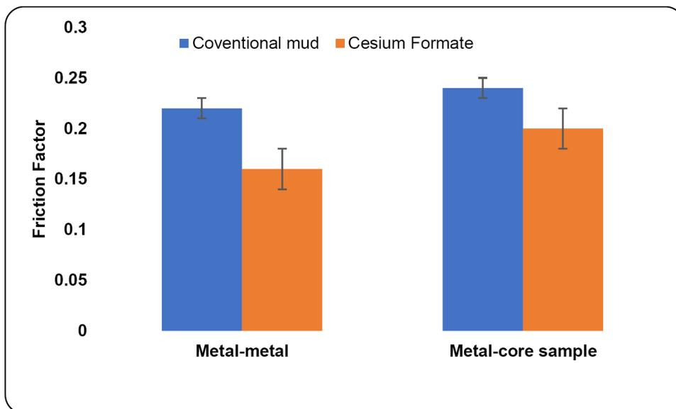
Figure 6—Friction factor profile of an inhibitive mud (Cesium formate) and a conventional water-based mud
