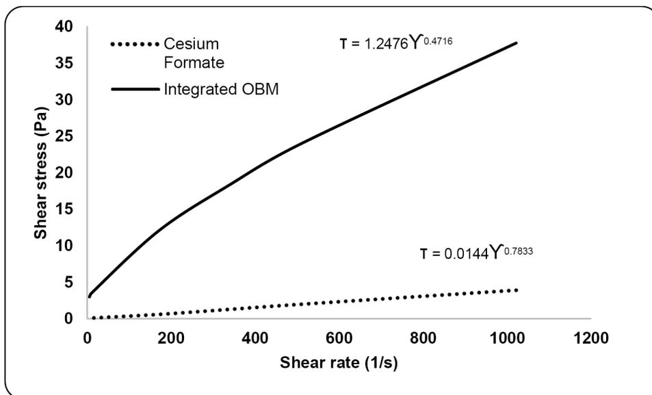
Figure 3—Shear stress vs. shear rate profile for integrated oil-based mud and cesium formate.
