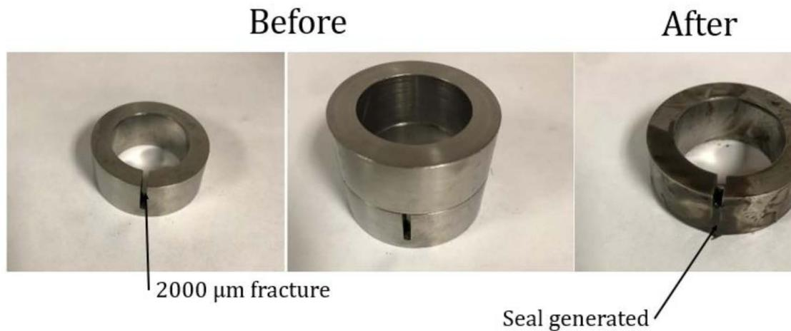
Figure 8—Disk slot before and after fracture sealing test.
