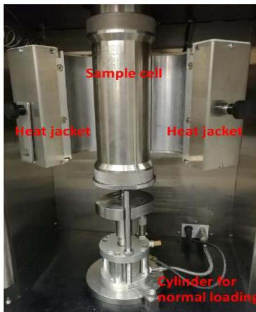
Figure 2—High pressure high temperature innovative dynamic lubricity tester
