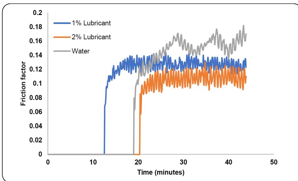
Figure 7—Effectiveness of lubricant in minimizing friction factor.
