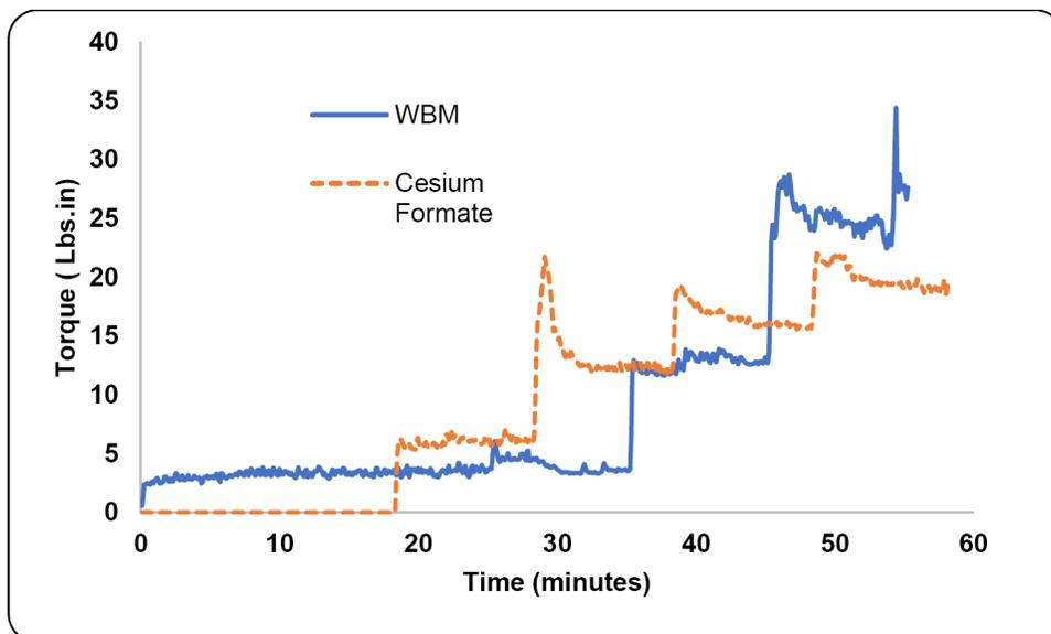
Figure 4—torque profile of an inhibitive mud (Cesium formate) and a conventional water-based mud.
